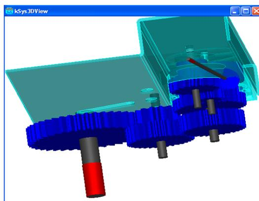
**Figure 1: Multi-stage Transmission with Casing Parts. The Transmission Stages must exactly fit in the pre-established Casing. The Casing Data will be read in STEP-format and displayed in the KISSsys 3D Window.**
