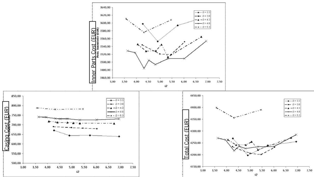
Figure 8: Cost of the inner Parts and total Cost (with Casing) for a Three-stage Helical gear gearbox depending upon the Transmission Distribution. Total Reduction  $i = 110$ ; Driving Torque 25 kNm at 9 rpm ( $i_3$ : Reduction of the Driving Stage,  $i_2$ : Reduction of the intermediate Stage).
