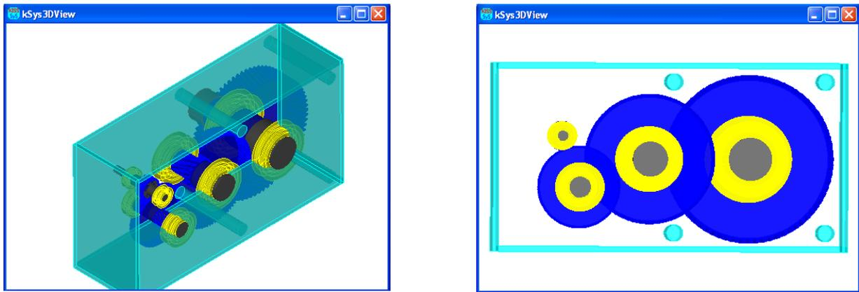
**Figure 5: Crane Gearbox showing the Space Constraints, given Position of the driving and driven Shafts and 4 Through-drills (Tubes). The Display comes from the first KISSsys Release in 2001.**
