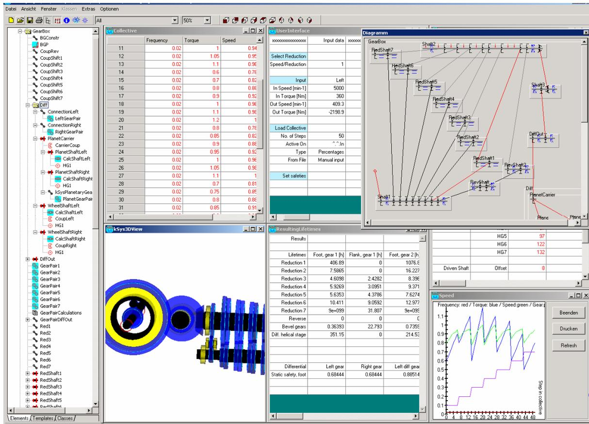
Figure 3.2-1 Views on the model. Left tree structure (logical structure). Top right: power flow. Bottom left: 3D view. In between: tables.
