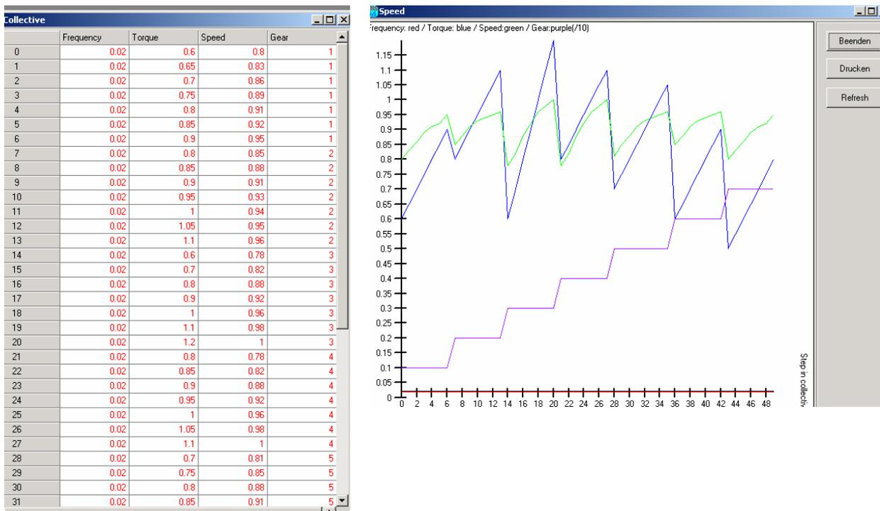
Figure 3.3-4 Left: load spectra in table form. Right: graphical representation (Due to confidentiality, values are fictive)
