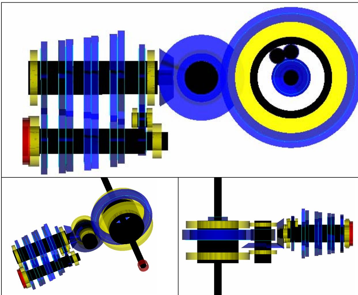
Figure 3.1-1 Structure of the gearbox: Black: shafts, blue: gears, yellow: bearings, red: power input or output. Of the differential only one pair of planets is shown.
